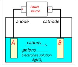
g) The electroplating cell is left running for 2.40 hours at a current of 2.35 amps and a voltage of 10.3 volts. What mass of silver is deposited in this time?
